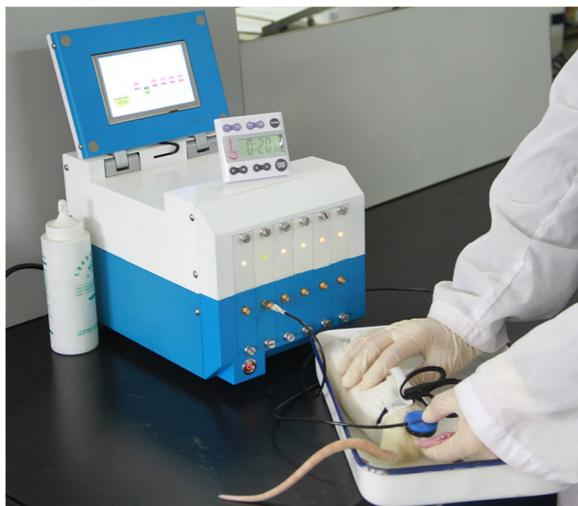
**Fig. 1** LIPUS instrument. The LIPUS device produced a 2000- $\mu$ s burst of 1-MHz acoustic sine waves repeating at 100 Hz with a spatial-averaged temporal-averaged (SATA) intensity of 30 mW/cm<sup>2</sup>. In the LIPUS group, the bilateral calf muscles of the rats were exposed to LIPUS for 20 min/day for 6 weeks
